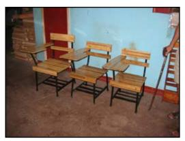
Sample chairs using engineered bamboo instead of wood produced by ADPI Cooperative in Iloilo City, Panay Island.
